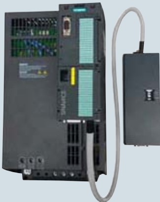
Chemical industry inverter comprising PM240 Power Module, CU250S-2 Control Unit and CM240NE chemical industry module
